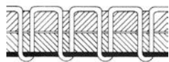
Fig. b: Needle-thread tension too low or hook thread tension too high
