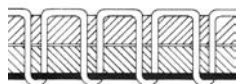
Fig. b: Needle-thread tension too low or hook thread tension too high
